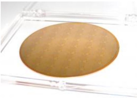
Figure 1: Power-supply transistors manufactured on a copper substrate
