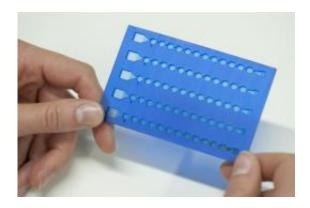
The magnetic nanoparticles transport the pathogen DNA into the detection chambers (on the right) on this plastic card. This is a prototype of the card for the fast sepsis test. Credit: Fraunhofer IZI
