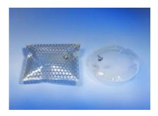
With a new gluing technique membrane cushions can be made in any geometry. Credit: Fraunhofer IFAM
