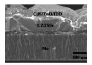
This image shows a cross-section of a CZTSSe thin film solar cell. The film exhibits densely packed grains, which leads to a high efficiency. Image credit: Qijie Guo, et al. ©2010 American Chemical Society.
