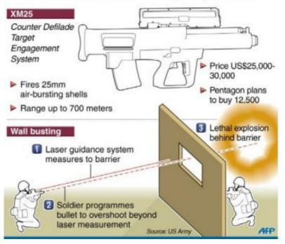
Graphic on the US army's new programmable "smart" gun that uses microchipped ammunition to target and kill enemy combatants hidden behind walls or other cover.
