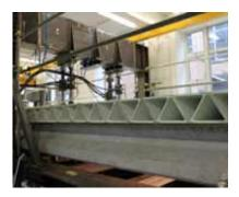
Triangulated glass fibre composite decking in Bristol bridge specimen. Image by Dr Wendel Sebastian
