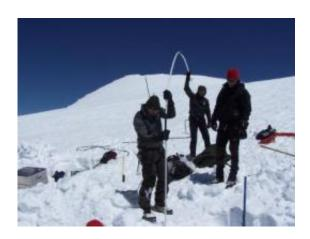
Researchers are installing an ablation stick, near a recently dug snow pit, to help in establishing the mass balance of the ice field. Credit: Paolo Gabrielli, Ohio State University
