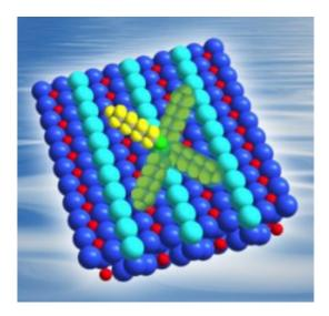
STM images of 1-, 2-, 3-, and 4-octoxy species anchored on TiO2(110) with corresponding models. The "X-like" appearance of 1-3 is a result of rapid rotational motion of alkyl chains among the equivalent surface binding sites. While 4 also rotates, its motion cannot be distinguished in the image from that of stationary species.
