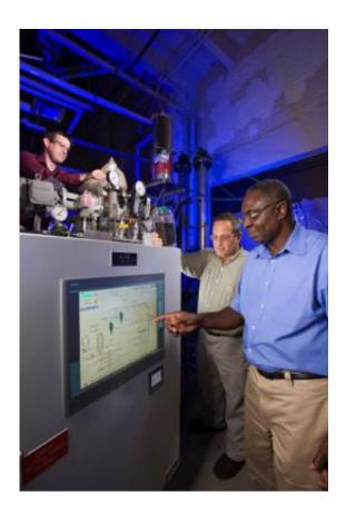
A team of ARS scientists including chemical engineer Akwasi Boateng (right), mechanical engineer Neil Goldberg (center) and chemist Charles Mullen (left) have made bio-oil by processing leftover barley byproducts with an intense burst of heat in the absence of oxygen. Click the image for more information about it.
