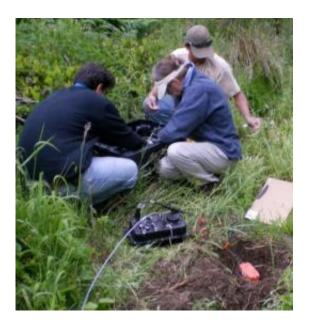
A seismic sensor (orange device) and datalogger (black box) are installed as part of one station in the "array of arrays" on the Olympic Peninsula in Washington state. The researchers are, from left, Danilo Galluzzo of Italy's Istituto Nazionale di Geofisica e Vulcanologia, Noel Barstow of the Iris/Passcal Instrument Center and Abhijit Ghosh of the UW. Credit: Lisa Foley, Iris/Pascal Instrument Center
