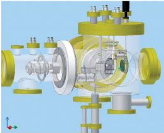
Figure 1: A schematic diagram of the antiproton decelerator at CERN that is used to smash antiprotons and molecular hydrogen molecules together so that the remaining particles can be analyzed to provide insight to their interactions. Credit: 2010 Helge Knudsen
