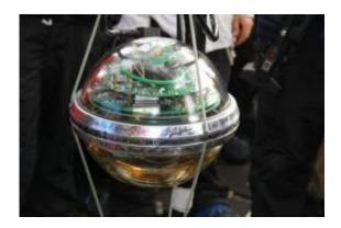
A handout picture taken on December 18 released by the US National Science Foundation (NSF) shows the final Digital Optical Module (DOM) which was to be deployed in the IceCube array, the world's largest neutrino observatory, built under the Antarctic tundra near the US Amundsen-Scott South Pole Station.
