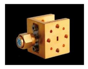
A THz mixer component containing a Schottky diode developed by Teratech Components Ltd.
