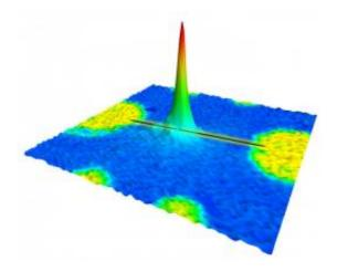
A microscope image of the light sensor shows the peaking photocurrent as it originates from the gap between the Etch A Sketch nanowires (in black). The Pitt researchers are the first to create a solid-state, oxide nanoelectronic device that combines electrical and optical capabilities onto one platform.
