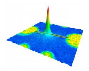
A microscope image of the light sensor shows the peaking photocurrent as it originates from the gap between the Etch A Sketch nanowires (in black). The Pitt researchers are the first to create a solid-state, oxide nanoelectronic device that combines electrical and optical capabilities onto one platform.
