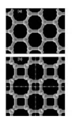
Views along [100]/[001], and [010] directions of 2x2x2 supercell of bct-Carbon,the dotted-dashed in (b) indicate the perpendicular graphene-like structure of bct-Carbon. Image credit: Xiang-Feng Zhou, http://arxiv.org/PS\_cache/arxiv/pdf/1003/1003.1569v4.pdf
