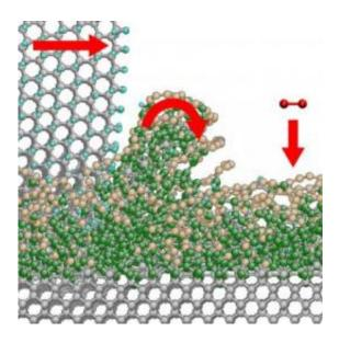
Material removal mechanism during diamond polishing: a sharp-edged diamond particle (gray atoms in the upper left) »peels off« a dust particle from the glasslike phase (green atoms) at the surface of the diamond (gray atoms in the lower part of the figure). At the same time, oxygen from the air (red atoms) reacts with the carbon chains (brown atoms) at the surface to form carbon dioxide. Credit: Fraunhofer IWM
