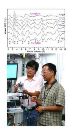
Top: Pair distribution function (PDF) of 16 nm-sized Y2O3 at high pressures. Bottom: Lin Wang (left) and Wenge Yang (right) of the Carnegie Institution of Washington shown with the diamond anvil cell and x-ray instrumentation used to probe the PDF of the sample at high applied pressures at room temperature.
