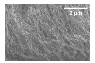
Fine hairs on the soles of gecko feet allow the lizards to climb vertical surfaces with ease. UA polymer researchers have discovered a synthetic glue (carbon nanotubes) with nearly four times the adhesion power of gecko hairs. Now the scientists reveal why the mimic version offers its remarkable staying power.
