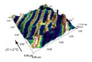
Theoretical research at Oak Ridge National Laboratory can help explain experimental results in vanadium dioxide, such as the formation of thin conductive channels (seen in white) that can appear under strain in a nanoscale vanadium dioxide sample.
