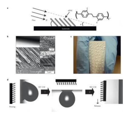
a, Schematic of PPX nanofilm deposition by OAP. b, Electron microscope crosssection of PPX nanofilm (insets show top view and high-resolution cross-section micrographs). c, Picture of the anisotropic adhesive wetting surface with water drops. d, Water adhesion and release in three configurations of the nanofilm. Schematics illustrate the nanorod inclination at each tilt angle and correspond to photographs showing the anisotropic wetting behaviour of the nanofilm. (Credit: Nature Materials)
