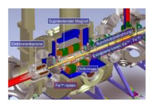
The researchers use EBIT, the electron beam ion trap, to reconstruct processes in the laboratory as they occur in the matter around black holes. Image: MPI for Nuclear Physics
