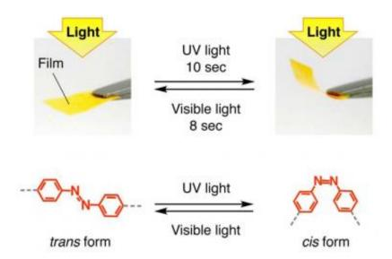
Top: Photomechanical bending motion of hot-pressed polymer brush film. Bottom: Structural deformation of azobenzene molecule upon exposure to UV and visible light.
