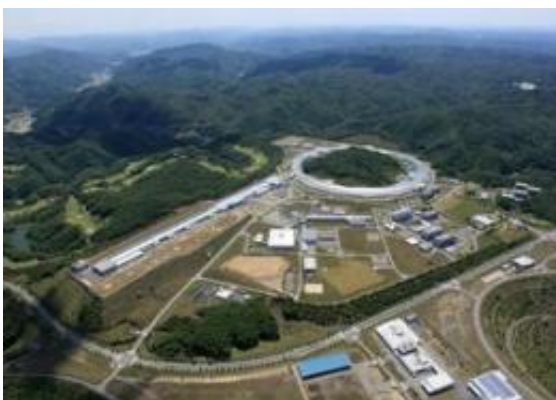
Figure 1: Aerial photo of the SPring-8 campus. The long structure extending diagonally to the bottom-left is the X-ray Free-Electron Laser (XFEL). To its right is the storage ring of the SPring-8 synchrotron. Copyright : RIKEN
