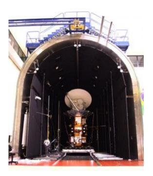
The joint U.S. and Argentine Aquarius/SAC-D spacecraft is prepped for thermal vacuum chamber tests at Brazil's National Institute for Space Research. Image credit: NASA/JPL-Caltech
