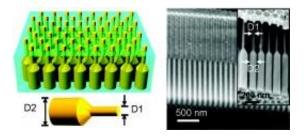
On the left a schematic of a germanium nanopillar array embedded in an alumina foil membrane; on the right are cross-sectional SEM images of a blank alumina membrane with dual-diameter pores; inset shows germanium nanopillars after growth. (Images courtesy of Ali Javey)
