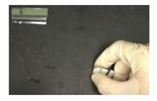
Compressing a nanogenerator between two fingers is enough to drive a liquidcrystal display. Credit: Courtesy Zhong Lin Wang
