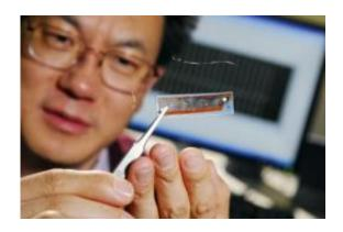
Professor Zhong Lin Wang holds an earlier version of the nanogenerators developed using zinc oxide nanowires. Credit: Credit: Gary Meek
