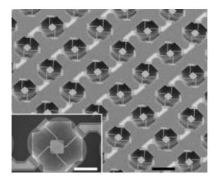
Illinois researchers developed an array of microsensors made of suspended platforms (inset) that can measure cell mass like tiny scales. Photo courtesy Rashid Bashir
