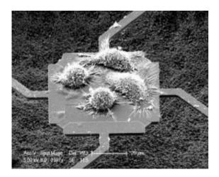
A scanning electron microscope image of cells growing on a microsensor. The researchers were able to measure the increase in mass as they watched a cell grow and divide into four cells. Photo courtesy Rashid Bashir
