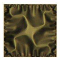
Top view, cathode side, of a free-standing Pt/YSZ/Pt fuel cell showing characteristic buckling patterns. The cell width is 160 microns. Photo courtesy of Shriram Ramanathan.
