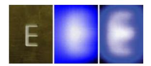
A typical sonagraphic image of the letter E etched into a copper plate reveals no detail (center). When evanescent waves from the object are captured and transmitted by the new 3-D holey-structured metamaterial, sufficient detail can be obtained to identify the letter. Credit: Jie Zhu/UC Berkeley, Johan Christensen/Universidad Autonoma de Madrid.
