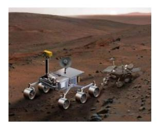
Comparison of Mars Science Laboratory and Mars Exploration Rover. The Mini Cooper-sized MSL rover is twice as long (about 2.8 meters, or 9 feet) and four times as heavy as the Spirit and Opportunity rovers. Credit: NASA
