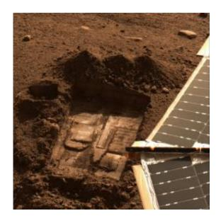
The Mars Phoenix mission dug into the soil of Mars to see what might be hidden just beneath the surface. Samples from this trench were delivered to the Wet Chemistry Laboratory, which was part of Phoenix's Microscopy, Electrochemistry, and Conductivity Analyzer (MECA). Credit: NASA/JPL-Caltech/University of Arizona/Texas A&M University
