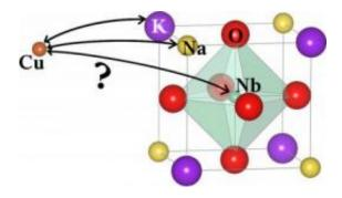
Computer simulation can calculate the possibilities of doping ferroelectric materials, such as potassium-sodium.niobate, with foreign atoms, such as copper. Credit: Fraunhofer IWM
