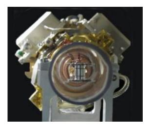
Installed and aligned symcap target inside its protective cover.
