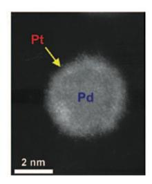
This high-angle annular dark field (HAADF) scanning transmission electron microscopy (STEM) image shows a bright shell on a relatively darker nanoparticle, signifying the formation of a core/shell structure — a platinum monolayer shell on a palladium nanoparticle core.
