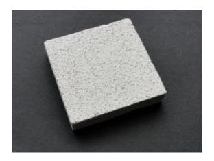
The new insulating plaster is simple sprayed onto walls. The photograph shows a block of the material.
