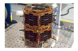
The FASTRAC satellites were built mostly out of aluminum and titanium. An orange, high-temperature tape called Kapton was also used.
