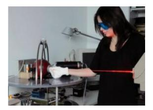
Measuring light losses in a polymer optical fiber.
