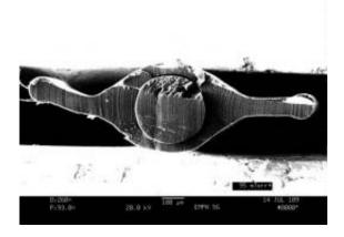
A bicomponent fiber imaged under the scanning electron microscope. The core of the fiber lends it the required stiffness whilst the sheath, of a different polymer material, gives it other desirable properties, for example optimal sliding properties.
