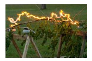
An electric arc created across a tree branch on an operating 7,200 volt operating distribution line at the PSAL test facility on the Riverside Campus at Texas A&M. Using computer based instrumentation, PSAL researchers have recorded the electrical characteristics of both staged and naturally occurring vegetation faults on operating utility systems.
