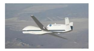
The Global Hawk can fly autonomously to altitudes above 60,000 feet. Image: NASA
