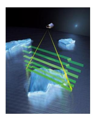
CryoSat can distinguish between altimetry signals returned from sea ice and open water - the difference between the two is known as the 'freeboard', and can be used to derive ice thickness. Credits: ESA /AOES Medialab
