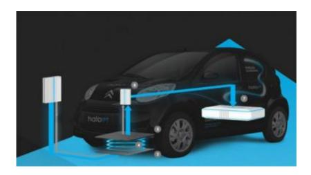
Wireless charging system allows the next generation of electric vehicles to be charged wirelessly. Credit: HaloIPT
