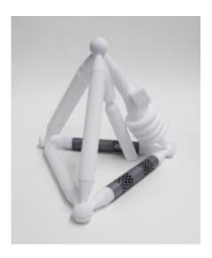
The robots consist of cylinder-shaped tubes with ball-and-socket joints that can assume different shapes depending on external factors and the purpose at hand. (© Fraunhofer IPA)
