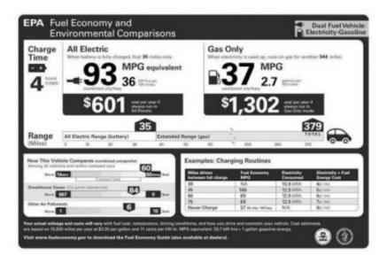
The combined estimate of 60 mpg makes assumptions on the frequency of recharging and on how much of the time a typical driver will be running the car on electricity and how much on gasoline. In practice a driver who plugs in the car every night to recharge the battery and who
