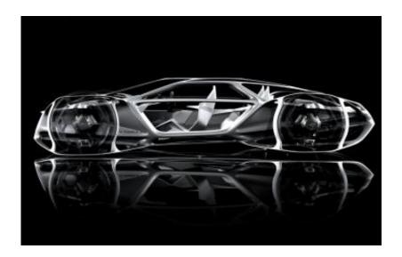
Additional technologies include an all-in-one wheel system that combines rotary actuator propulsion, steering and suspension functions. A drive-by-wire system decreases the mass of electrical components, while vehicle-to-vehicle communication promotes active safety.
