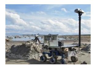
JPL's prototype sample-collecting rover drills into a rock along the shore of Mono Lake. Credit: Henry Bortman
