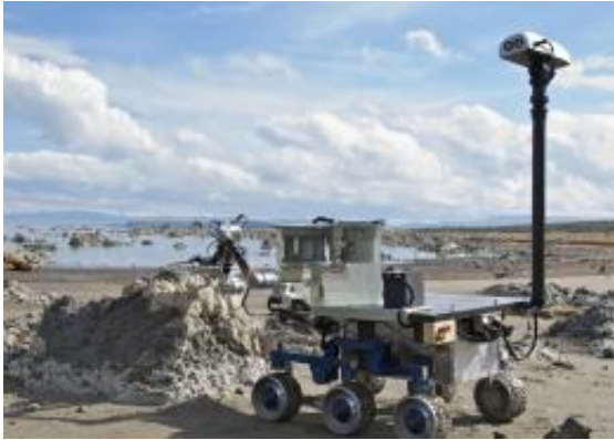
JPL's prototype sample-collecting rover drills into a rock along the shore of Mono Lake. Credit: Henry Bortman
