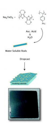
Using simple water-based chemistry to wrap a polymer that conducts electricity around a nanorod of tellurium, this composite nanoscale thermoelectric is easily spin cast or printed into a film.
