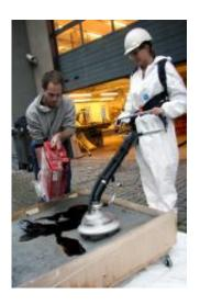
Cleaning up oil spills is a time consuming, difficult process. But a novel approach developed at the Norwegian University of Science and Technology (NTNU) uses a new kind of vacuum cleaner that blows bark or other absorbent material onto oil spills, and then sucks the material up again. The vacuum cleaner is four times more efficient in cleaning up after oil accidents than conventional techniques.
