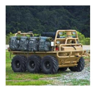
The SMSS Block 1 is the newest variant, featuring a lighter frame, upgraded sensors and better accessibility.
