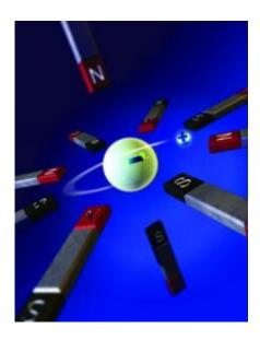
An octupole magnet was critical to trapping antihydrogen atoms by using their small magnetic moments. This simplified version shows how the north and south poles of strategically arranged magnets can immobilize a neutral antihydrogen atom that has a magnetic moment equivalent to a tiny bar magnet. Credit: Katie Bertsche
