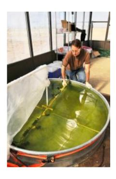
Algae is considered a prime candidate to serve as feedstock for biofuels because of its high energy content and yield, rapid growth and ability to thrive in seawater or wastewater. Oil from algae can be refined into gasoline, biodiesel or jet fuel. Credit: Photo courtesy of Sandia National Laboratories
