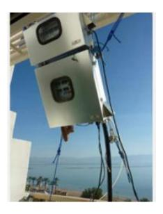
Instruments for measuring atmospheric mercury are on a balcony facing the Dead Sea. Credit: Daniel Obrist
